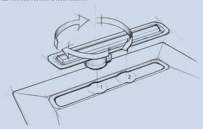
The drain outlet is offset allowing the drain to be rotated 180° at installation, the outlet is also fully rotatable allowing 360° waste positioning to avoid any potential obstacles such as joists and pipework.
