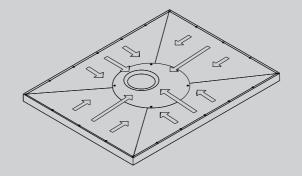
Offering the most versatility and size options, the central drain plate of the Aqua–Dec EasyFit can rotate 360° to avoid all underfloor wetroom obstructions and can be trimmed anywhere up to the solid surround. This floor former can be used with a variety of drain types to suit all applications, and a range of Drain Tops to add individual style to every wetroom. The Aqua–Dec EasyFit is 22mm thick and can be installed on timber or concrete floors, providing flow rates of up to 36l/min.
