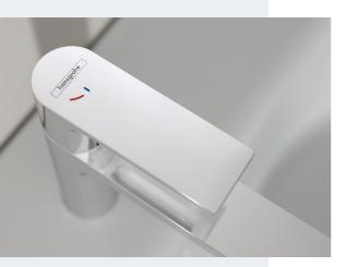
AirPower technology enables our mixers to use as little as 4.5 l/min whilst maintaining great performance. By drawing in the air via the jet outlet it enriches the incoming water, making the jet fuller, lighter and softer. Delivering a high jet volume with less water.
